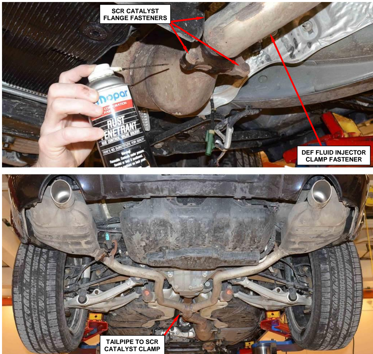
Figure 3 – Saturate Exhaust Fasteners with Penetrating Lubricant
