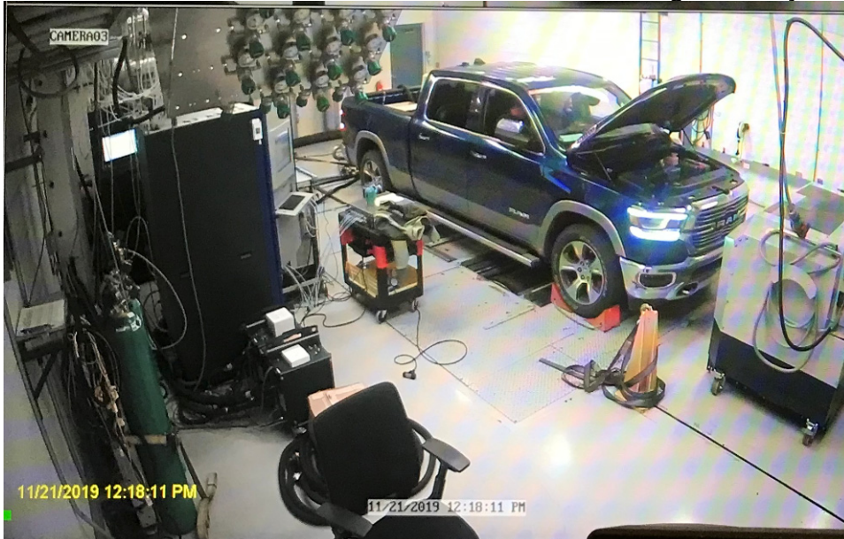
Correlation of Sensors, Inc. PEMS to Mahle modal and bag bench Dynamometer
