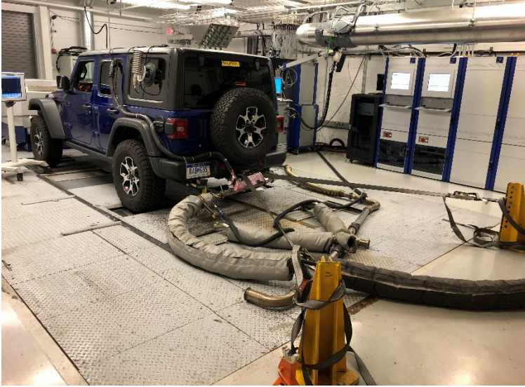
Correlation of Sensors, Inc. PEMS to Mahle modal and bag bench Dynamometer
