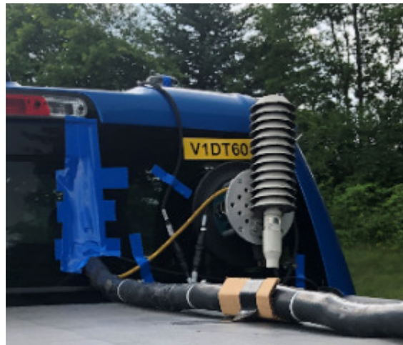
Figure 13 - FCA Vehicle Tag, Weather Probe and GPS
