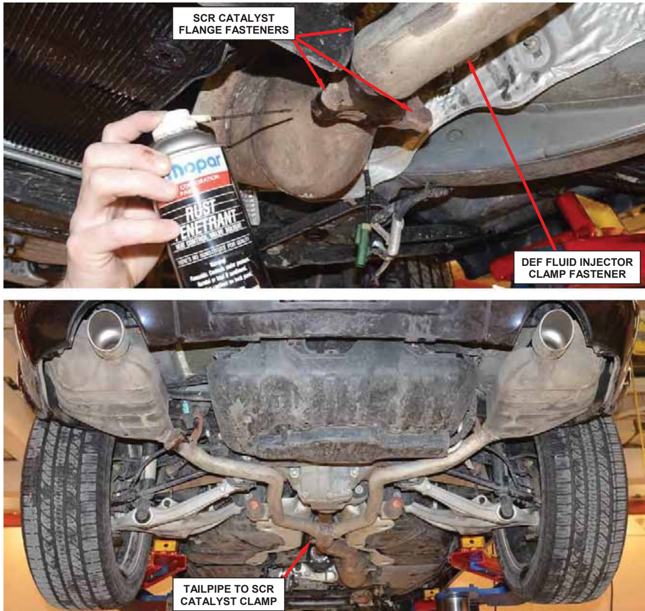
Figure 3 – Saturate Exhaust Fasteners with Penetrating Lubricant
